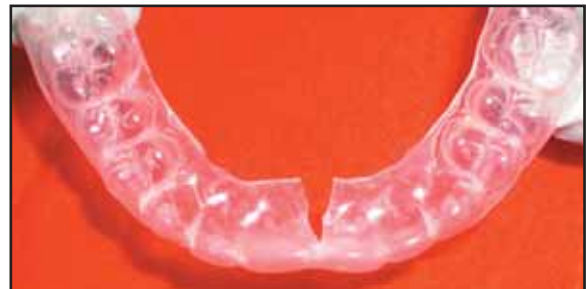
Fig. 4 Fragility of type "A" plastic evidenced by torn and cracked thermoplastic retainers.
